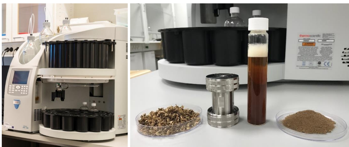
Figure 9. ASE-350 Accelerated Solvent Extractor (Thermo Electron Sweden AB, Hägersten, Sweden) on the left. Dried BSG, sample cell used in ASE-extractions, alkaline extract and pH-shift precipitated and dried proteins enriched extract on the right.
