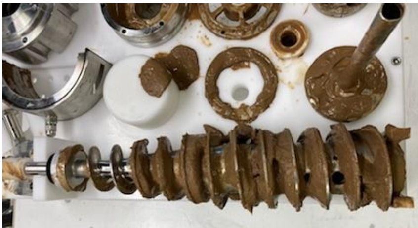
Figure 5. Buildup of proteins enriched fraction inside the screw conveyor of the decanter centrifuge during the separation process.
