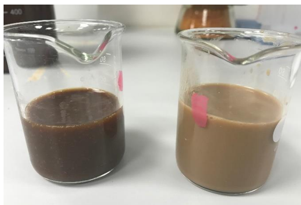
Figure 6. Dark brown alkaline slurry from the pilot scale extraction after the first centrifugation on the left and pale brown precipitated proteins enriched slurry after pH adjustment of the slurry on the left to 3 on the right.
