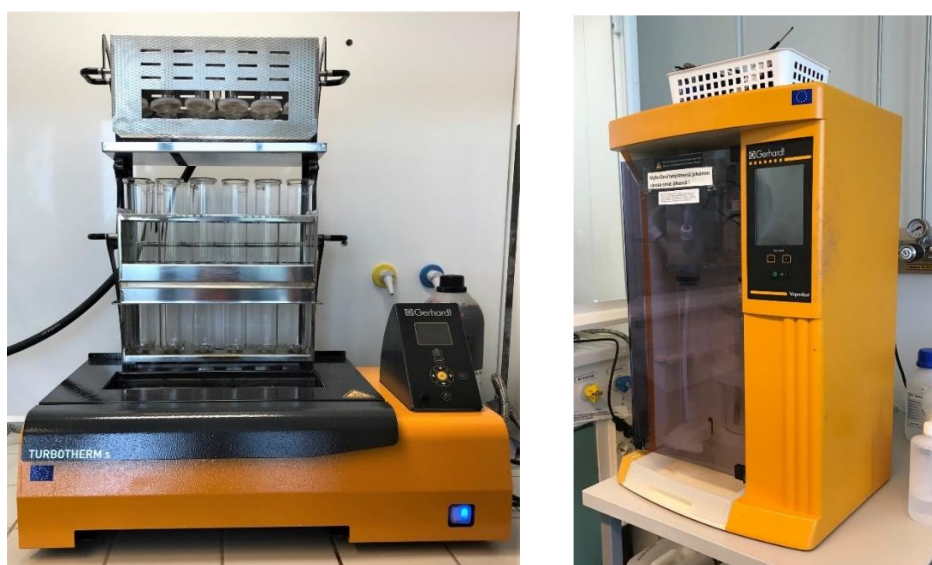
Figure 2. TURBOTHERM Kjeldahl digestion block (C. Gerhardt GmbH & CO. KG, Königswinter, Germany) on the left. VAPODEST distillation system (C. Gerhardt GmbH & CO. KG, Königswinter, Germany) on the right.
