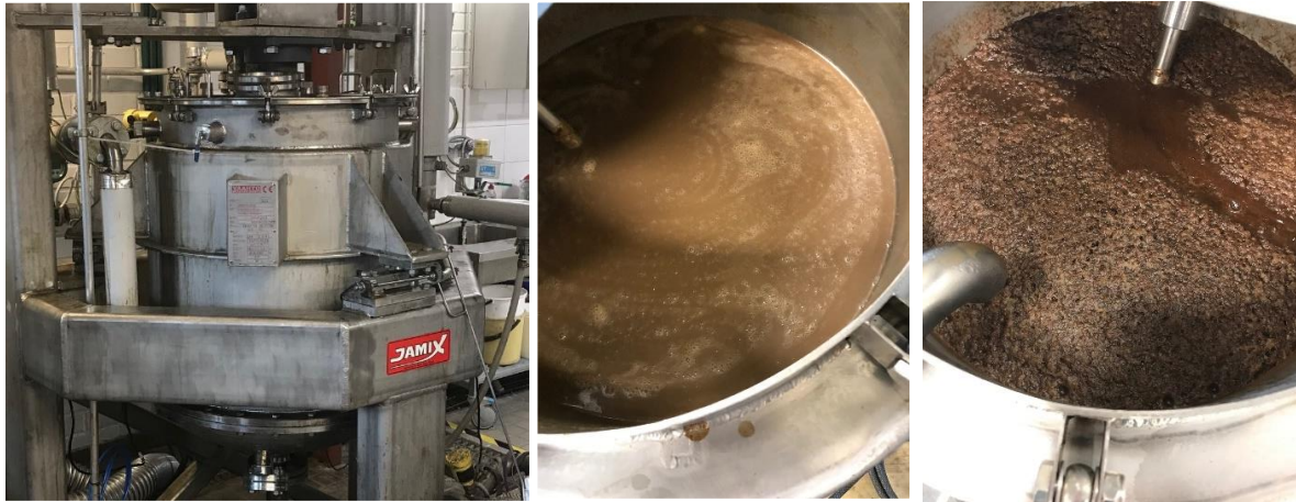
Figure 3. Pilot scale extraction in 200 L batch reactor. Reactor on the left, dilute acid treatment in the middle and alkaline extraction step on the right.
