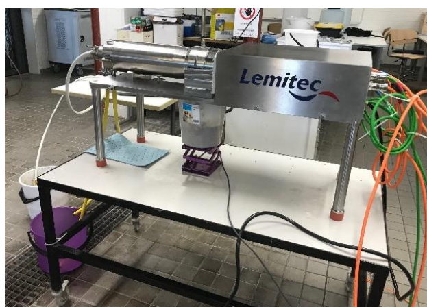
Figure 4. Lemitec MD 80 decanter centrifuge used in separations of solid and liquid matter after large scale extractions on the left. On the right: section view of a 2-phase decanter centrifuge.
