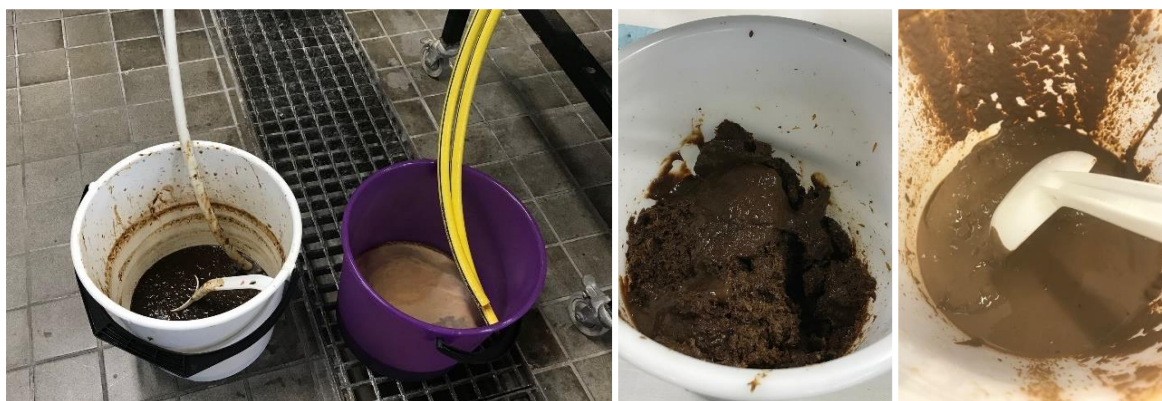
Figure 8. On the left: in white bucket BSG slurry after the extraction and in purple bucket liquid containing soluble material after the centrifugation. In the middle: residual BSG after the separation. On the right: protein-enriched fraction after pH-shift of the liquid in purple bucket and separation of the precipitated proteins together with other solid matter in decanter centrifuge.
